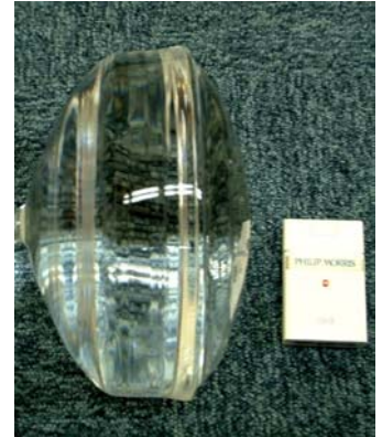
Fig.1. 8-inch size \text{CaF}_2 single crystal grown by the Cz technique. This crystal was grown in collaboration with Tokuyama Corporation.
